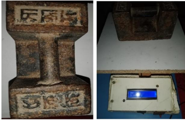
Figure 8. Weight Verification By 5 kg Known Weight.
